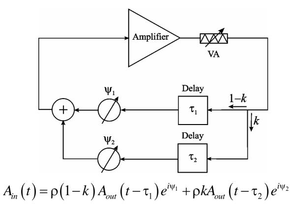
k — control parameter,  $\rho$  — attenuation produced by the VA
