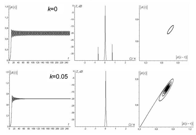
According to derivations presented above we must choose  $\tau_2=2.43$ ,  $\psi_2=2.02\pi$ Adding of the secondary control feedback allows to suppress self-modulation
