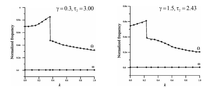
Fundamental frequency does not depend on *k* while the modulation frequency switches to the frequency of another mode at  $k \approx 0.3$
